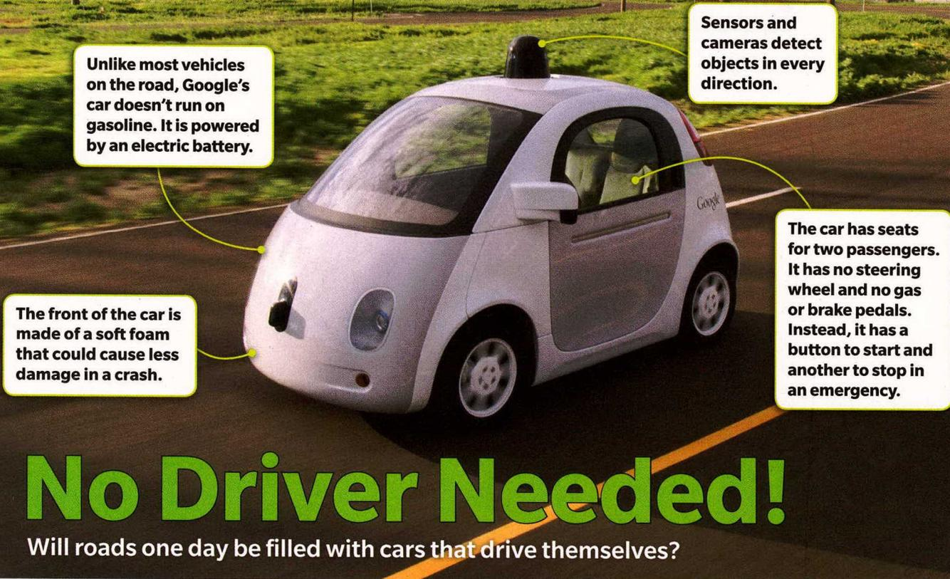
Unlike most vehicles on the road, Google's car doesn't run on gasoline. It is powered by an electric battery.
